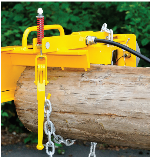
Chain Binder mount for wooden poles only.
