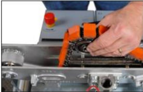
7. Remove the tension sprocket assembly
