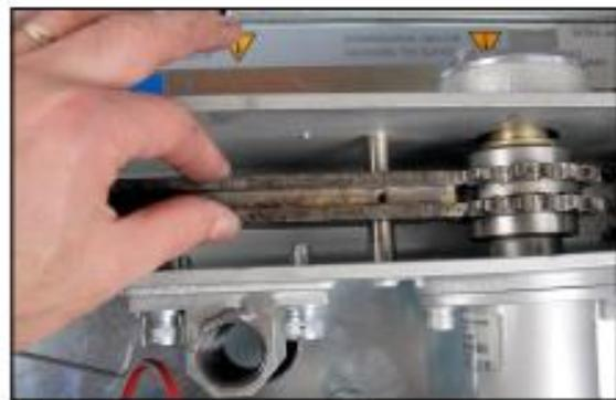
10. Check the chain support slide bars for wear. Clean and relubricate.
