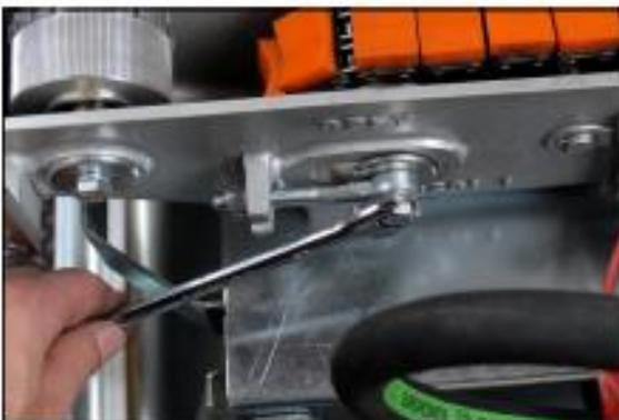
5. Remove the swing bolt from the side of unit using a 13mm wrench.
