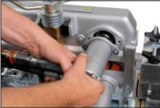
1. Remove the hydraulic motor from the top frame using 6mm Hex Key. Do not disconnect hydraulic hoses connected to the motor.
