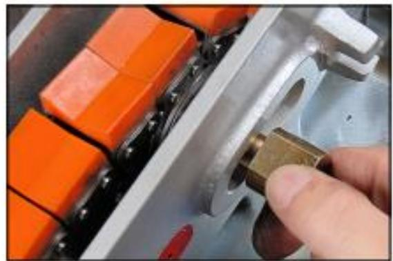
6. Pull the tensioner pin out from the sprocket assembly. Remove spacer from other side.
