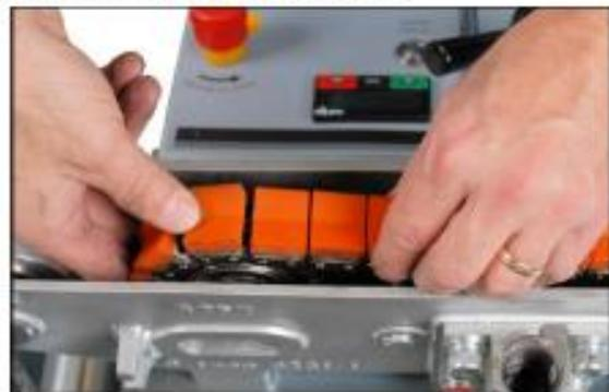
12. Align the tension sprocket with the chain and locate into position. Insert the tension pin through the tension sprocket. Place the tension pin spacer on the tension pin through the opposite hole. Refit swing bolts using a 13mm wrench. Adjust the chain evenly via the swing bolts, checking free rotation of the chain. Do not over tighten the chain.
