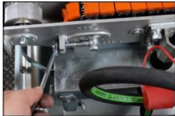
4. On the lower unit, slacken the 2 chain adjusters using a 13mm wrench.
