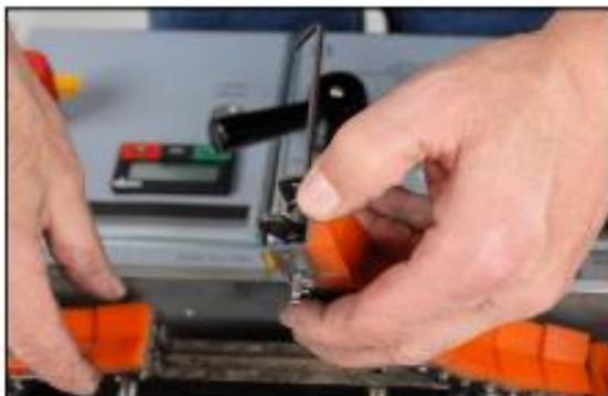
11. Pass the pre-lubricated new chain around the drive sprocket. Feed the chain along the unit and reconnect the chain-connecting link. Remember to install the 2 center connecting link plates.
