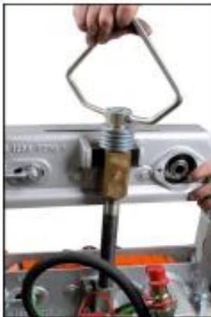
3. Unscrew the main clamping screw and separate the top and the bottom of the pusher unit. Place in a safe location.
