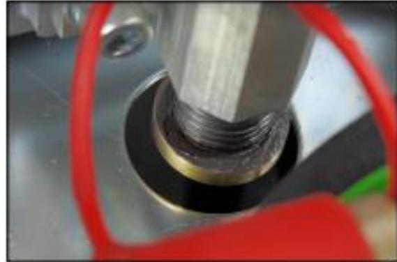
2. Remove the stop washer on the bottom of the main jacking screw using a 6 mm Hex key.
