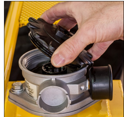
Indicator showing need for filter element replacement.
