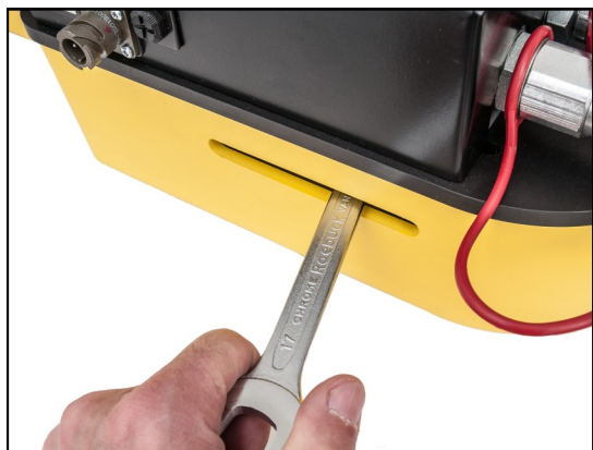
Loosen lock nut on pressure relief valve
