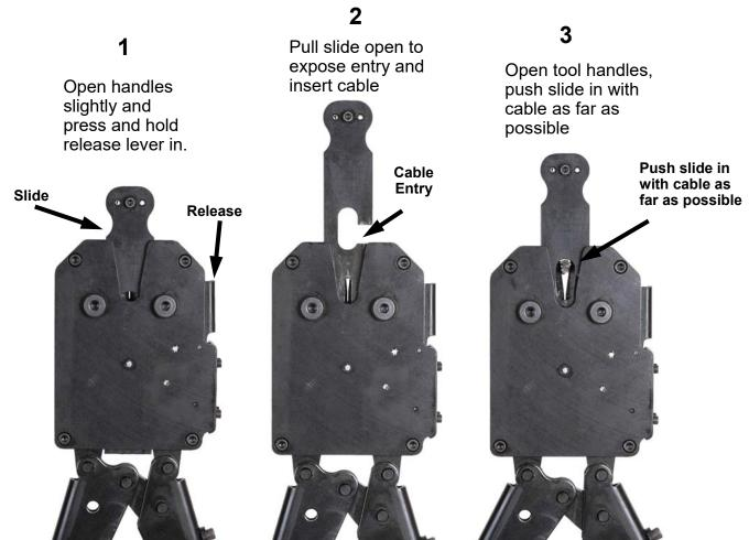
Open (wide) & close handles listening for ratchet click to cut cable. The ratchet mechanism will then pull the cable with each click into the tool until cable is cut.
