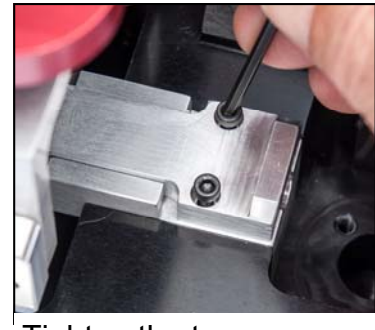
Tighten the two screws retaining the top plate of the air-box in-feed guide.
