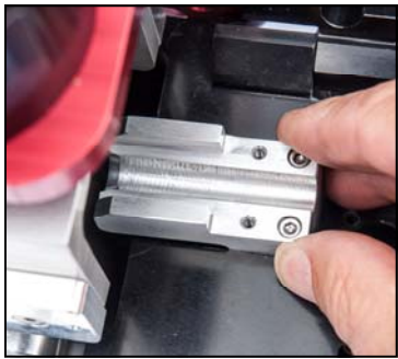
Place the guide in the groove on the exit side of the roller
