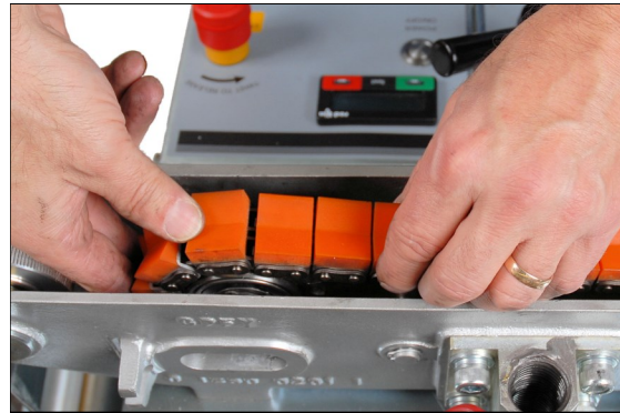
10. Check the chain support slide bars for wear. Clean and relubricate.
