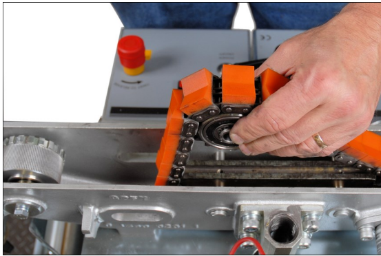
7. Remove the tension sprocket assembly
