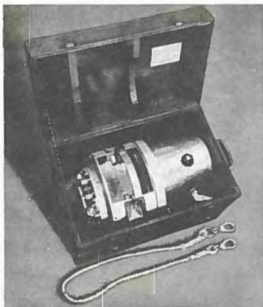
Pulling plate gate should be all the way open and the drum in the locked position before placing the lasher into its case. *Keep the lasher in the carrying case at all times when not in use.*
